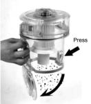
After you have emptied the dust container, hold the HEPA filter from the stem and twist it counter clockwise to release it from the dust cup container.
